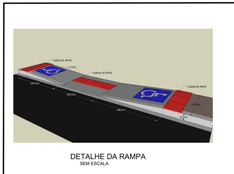
DETALHE DA RAMPA SEM ESCALA
